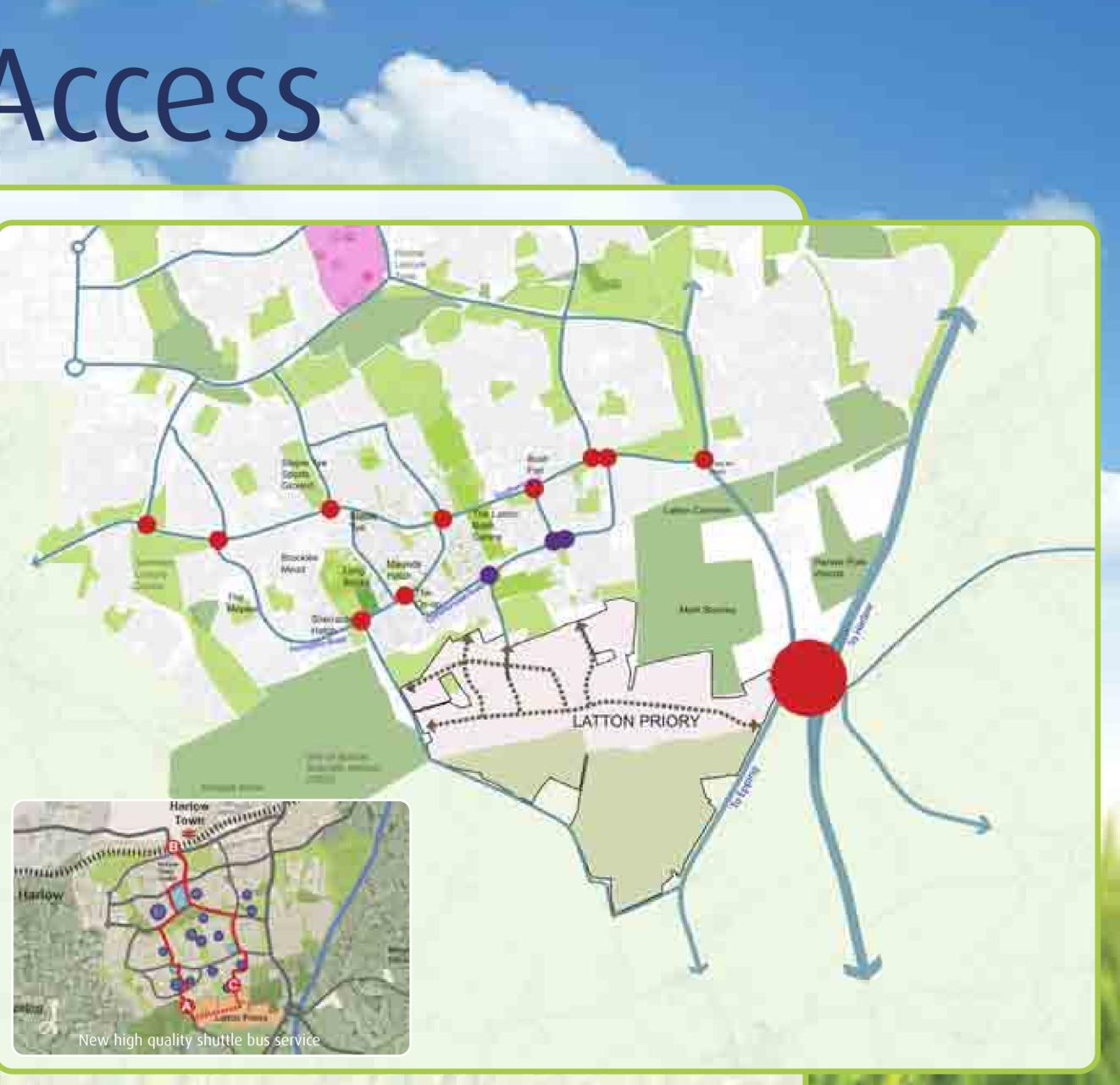
Potential vehicle connections showing the key junctions which are being considered as part of an improvement/capacity study
